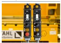
The two-step SWH Ex control pendants in IP 66 protection are used on explosion-protected wire rope hoists for Zone 1.
