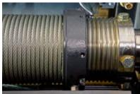
The wear-resistant rope guide in nodular graphite casting GJS (previously designated GGG) is extremely durable and not subject to temperature limitations. The same applies to the chain guide, type of protection used: constructional safety >cc.
