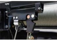
The overload cut-off operates with a dual channel load sensor supplying analog signals. Various sensors are used depending on reeving (LCD, LSD).
