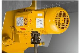
The explosion-protected travel drives Zone 1 and Zone 21 are designed for intermittent operation. They have a sliding rotor motor with conical brake and centrifugal mass for smooth starting and braking characteristics. All motors are pole-changing providing two travel speeds. The particularly quiet gear requires little maintenance thanks to its long-term oil bath lubrication.
