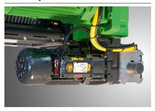
Crane systems up to a safe working load of 50,000 kg and a span of 30 m can be built with explosion-protected endcarriages for underhung and overhead travelling cranes. For particular applications, at customers' request and for increased safety all wheels can be supplied in brass.
