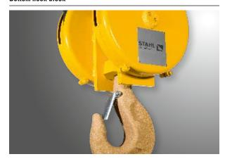
For high and very high travelling speeds the load hook and the solid parts of potential impact surfaces are bronze-coated. In addition, all other exterior surfaces of the bottom hook block can be bronze-coated to prevent sparking.
