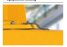
Equipotential bonding is essential for avoiding incendive sparks when installing crane technology in potentially explosive atmospheres.
