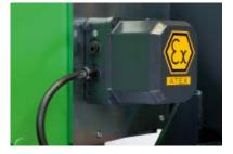
The protection class of the gear limit switch is IP 66. The elements installed are protected by flameproof enclosure >d<, the housing by increased safety >e<.
