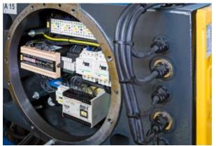
Flameproof enclosure for Zone 1 and Zone 2: the sheet steel or aluminium housings can be used as individual housings or in combination. All components required such as transformers, contactors, fuses, measuring instruments and tripping devices can be installed in the modular-design housing. Post-type bushings provide the connection to the terminal box (in increased safety Ex e).
